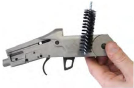
17. Oil the inside and outside of the frame. Be sure to oil all metal surfaces.
