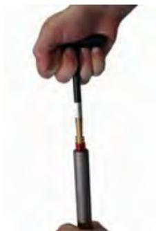
5. With the concave end of the loading jag on your ramrod, position the ramrod on top of the bullet inside the bore. Holding the ramrod no further than 6" over the bore, apply firm pressure downward until the bullet is seated against the powder charge. (Holding the ramrod higher will increase your chances of breaking your ramrod.)
