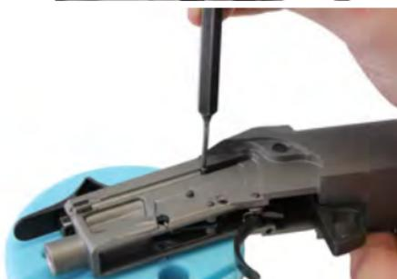
7. Depress the Barrel Catch lever to remove the Striker Assembly. Remove from rear of the frame.
