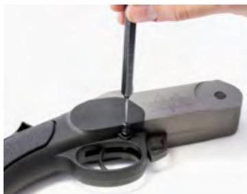
8. Press the barrel catch lever in and reinstall the barrel assembly onto the frame and lock into place.
