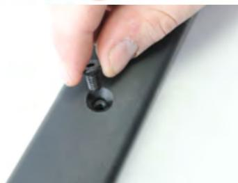
11. Reinstall the Accelerator™ Breech Plug. Note: Before attempting to install the Accelerator Breech Plug™ be sure to inspect the fire channel of the breech plug to make sure it is clean and free of any obstructions.
