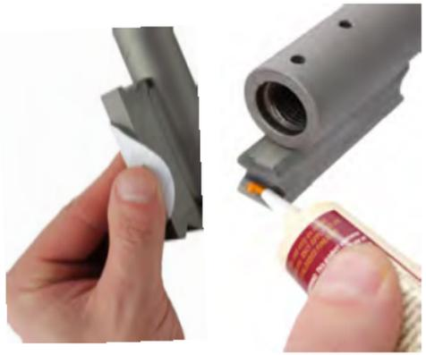
14. Apply a light coating of gun oil to the outside of the barrel and all metal surfaces including the extractor.
