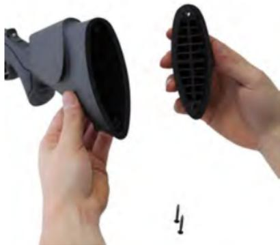
3. Remove the stock bolt and stock bolt washer using a 6mm Allen key socket, 8" socket extension, and standard length socket ratchet by turning counter clockwise to loosen the stock bolt and remove.
