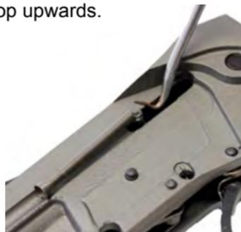
6. Completely remove the Striker Retention Spring Pin from the frame using a small punch and rubber mallet. Tap the pin out from right to left.
