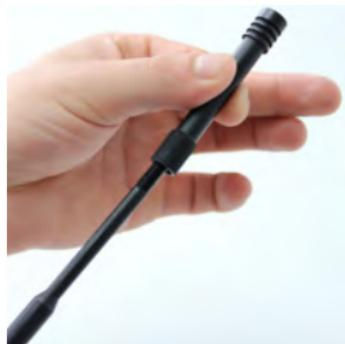
5. Insert the ramrod into the barrel. When it is touching the top of the breech plug it should sit approximately 3/4" below the muzzle.
