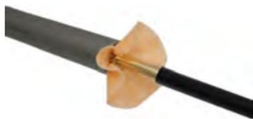
13. Lightly spray the barrel lug with Traditions® Cleaning Solvent. Wipe the solvent off with a dry cotton cleaning patch. If these areas are heavily fouled use the nylon brush to help remove fouling from the barrel catch and pivot points.
