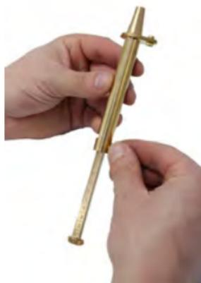
3. Pour powder from your Traditions® flask into the powder measure. Pour powder from the powder measure down the barrel.
