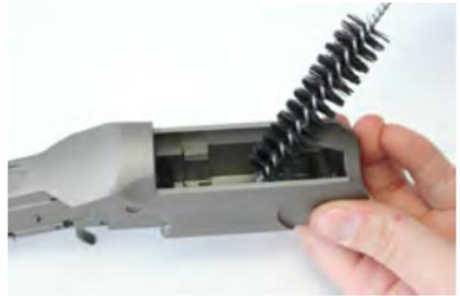
16. To clean the outside of the frame, lightly spray it with solvent. Use the Nylon Brush to remove any fouling from the outside of the frame, the barrel release lever, hammer, hammer extension, and inside the hammer channel.
