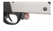
Your Traditions rifle is equipped with a trigger block safety & a hammer block safety. The hammer block safety is designed to prevent a misfire if the hammer were to fall without being engaged by the trigger mechanism.
