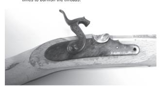
Test that the trigger moves freely within the trigger guard. If not, move it back & forth a few times to free up any binding. Pushing the trigger sideways in its housing will also help loosen its movement.
